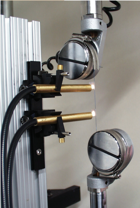
Figure 1, Strain Controlled Wire Fatigue Experiment.
