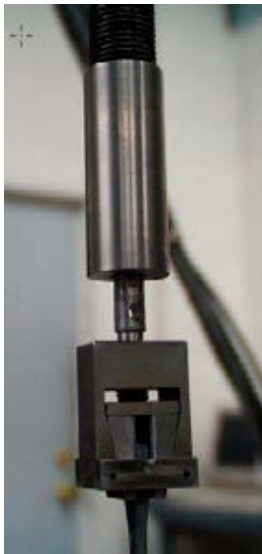
Figure 26, High strain gripping system allows the system to achieve a high speed before engaging the specimen.
