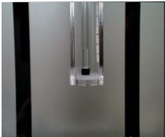
Figure 29, A black plastic disk specimen rests between glass platens in a thermomechanical analysis test instrument in advance of a thermal expansion experiment.
