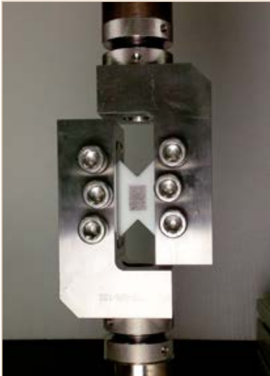
Figure 15, Rail shear specimen installed with DIC pattern.
