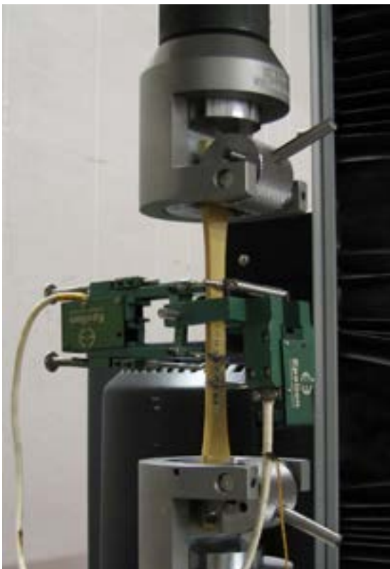
Figure 8, A tensile specimen with an axial extensometer and a transverse extensometer mounted.
