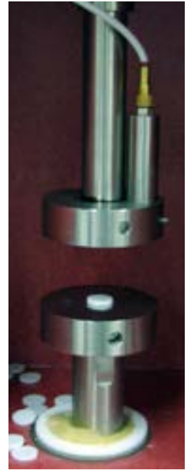
Figure 14, Compression platens with capacitive strain sensor.
