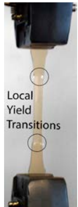
Figure 12, Localized yielding or necking in the tensile specimen - making it difficult to understand the distribution of stress and strain in the test specimen.
