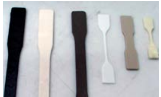
Figure 4, A variety of standard plastic tensile specimens
