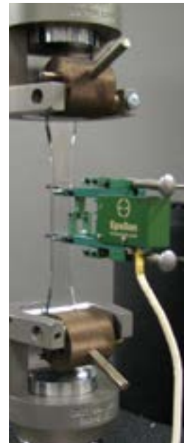
Figure 2, Plastic tensile test with an axial extensometer mounted to the specimen.
