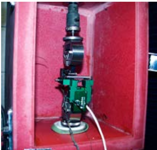
Figure 27, A tensile specimen with axial and transverse extensometers mounted on a test specimen in an environmental test chamber.
