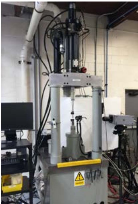
Figure 25, A high energy high strain rate test system.
