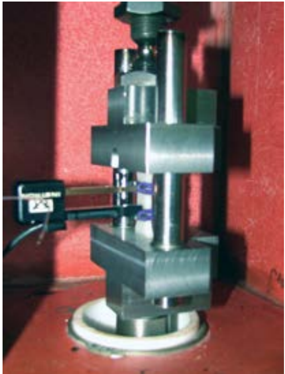
Figure 18, The in-plane compression fixture is used to support compressive straining in the plane of the material sheet. This can be used for creep tests of low strain compression.
