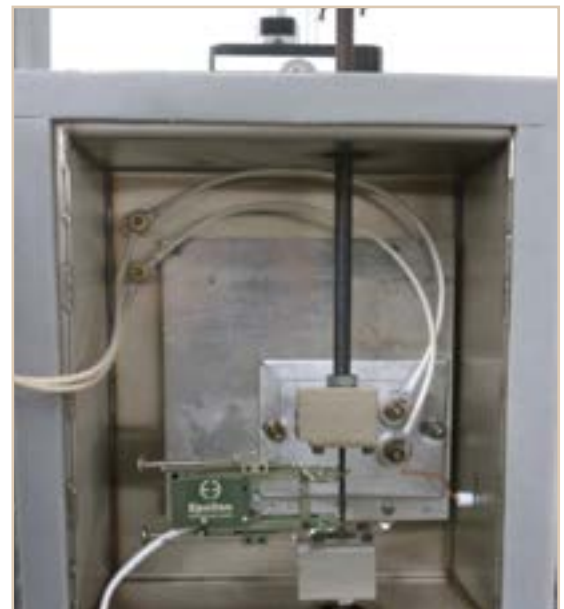
Figure 23, Plastic tensile specimen with extensometer (green) mounted inside the temperature chamber of a creep frame.
