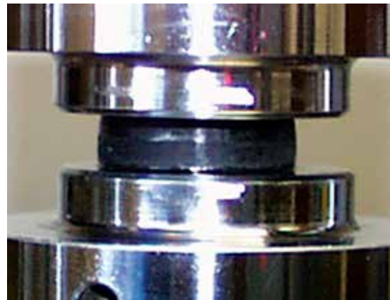
Figure 6, A Lubricated Compression Specimen Showing Lateral Constraining from Friction at the Surface
