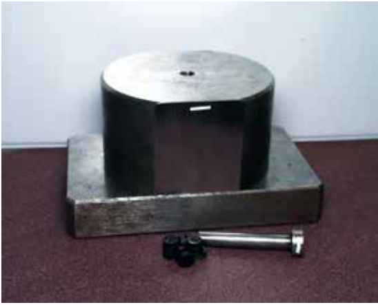
Figure 9, A Volumetric Compression Fixture with Specimens
