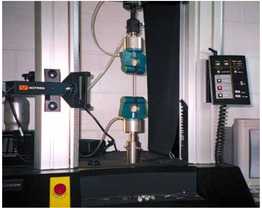
Figure 3, A Tension Experiment using a Video Extensometer
