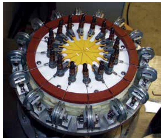
Figure 8, A Biaxial Extension Experiment using a Laser Extensometer (Out of the Image)
