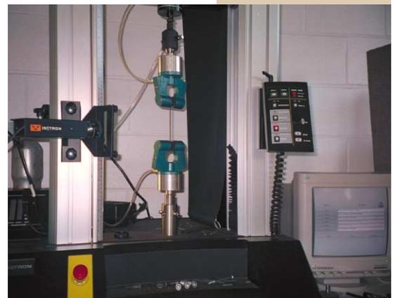
Figure 10: Simple Tension Test with Video Extensometer
