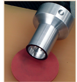
Figure 9, Axial Torsion Friction Experiment Material Specimens Aluminum and Rubber
