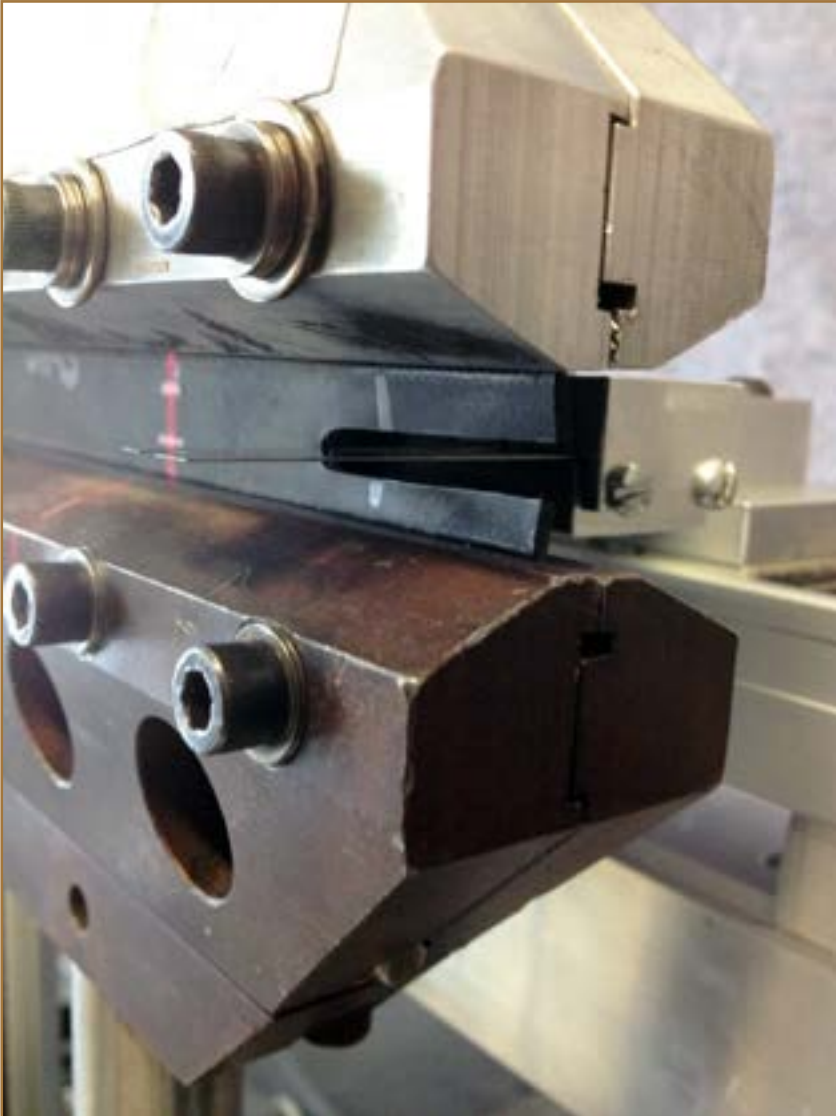
Figure 1, Sharpened Blade Contacting a Pre-strained Specimen
