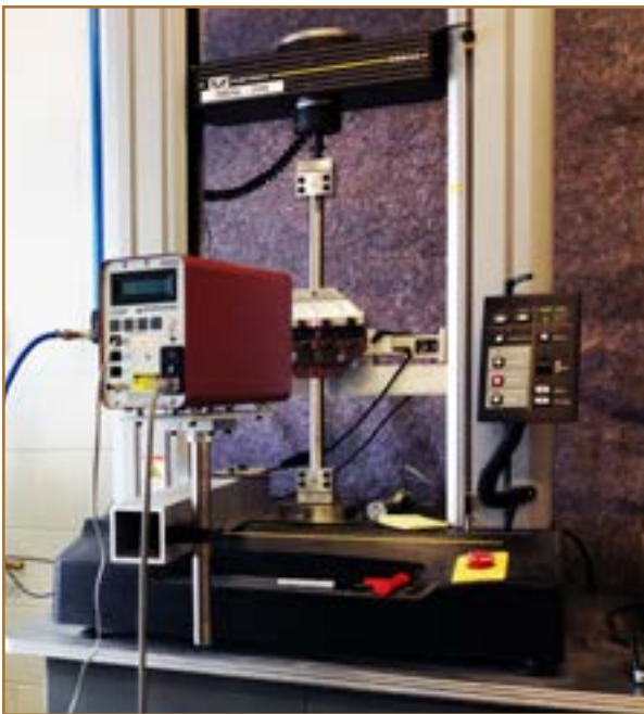
Figure 3, Complete Cutting Resistance Instrumentation
