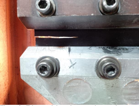
Figure 2. Edge crack in a planar tension specimen.
