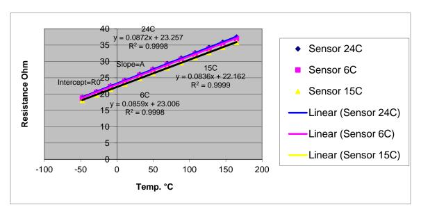
Range of  $A \sim 0.20 - 0.30$  Ohm/°C depending on sensor design Range of  $R_0 \sim 60 - 70$  Ohm
