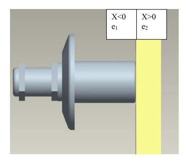
$$\Delta T_1(x,t) = \frac{2G\sqrt{t}}{e_1 + e_2} ierfc \frac{|x|}{2\sqrt{a_1 \cdot t}} \text{ for } x < 0, \ t > 0$$
